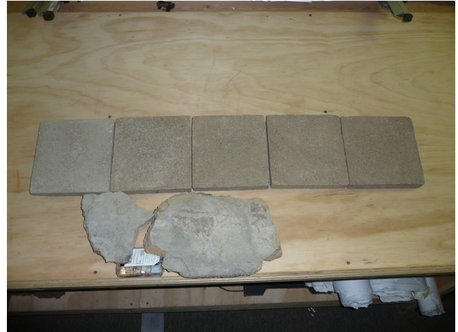
Various concrete mix sample designed to match the original architectural concrete, shown in the foreground. Note the different degrees of buff color in the mixes.
